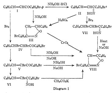
given to the formation of the isoxazoline (III) from benzal-*p*-bromoacetophenone (I) and its oximes (II), and to the formation of the isoxazole (VIII) from the dibromide of benzal-*p*-bromoacetophenone (IV) and its oxime (VII). The reactions involved are shown in diagram I.
